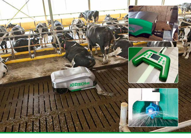
The JOZ-Tech manure robot is a fully-automatic robot for cleaning dairy cattle stables. Due to its high capacity the floors are clean and the cows experience a higher welfare.
